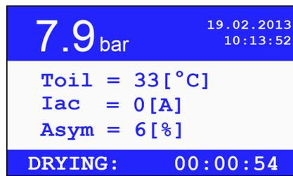
Figure 11: View of the MS-485 screen with the drying function turned on.
