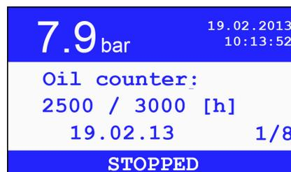
Figure 3: View of the oil counter screen.
