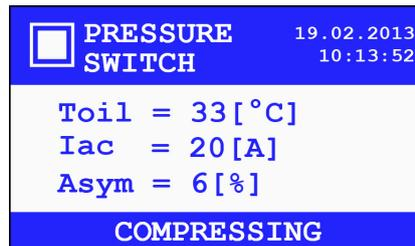
Figure 12: View of the MS-485 screen with the pressure switch function turned on
