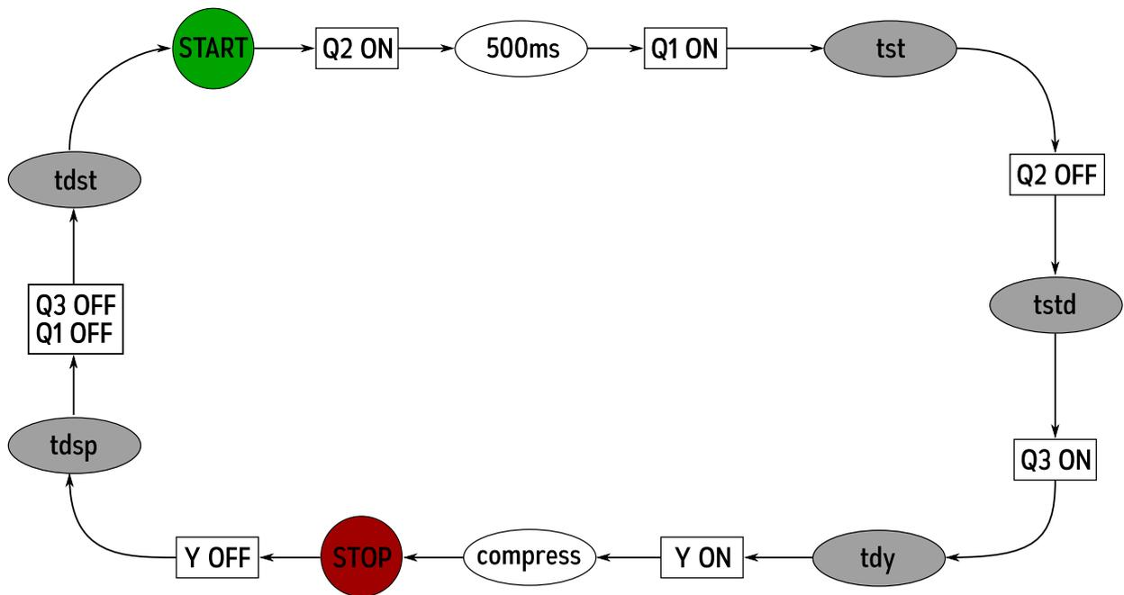
Figure 4: Motor control diagram
